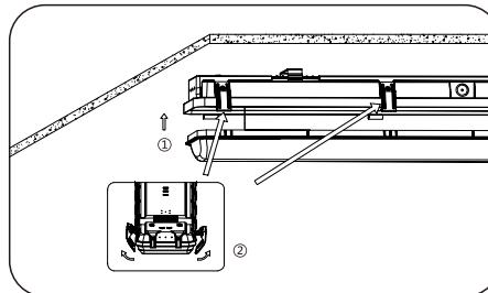
6. After align lens and bottom housing, turn off the luminaire. Secure lens to housing with lens latches.
