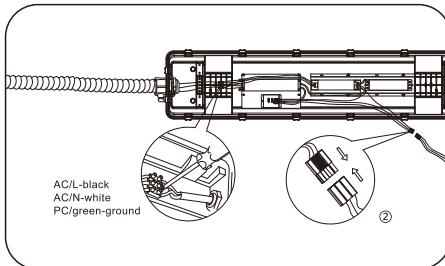
5. After the connection is completed, tighten the waterproof plug. Reconnect the wiring between the LED board and the driver.
