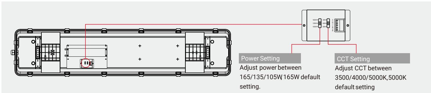
Note: Before Setting Power & CCT, release latches by pulling top of latch away from housing. Gently squeeze the buckle in and take out the PCB board (be careful not to touch the LEDs)
