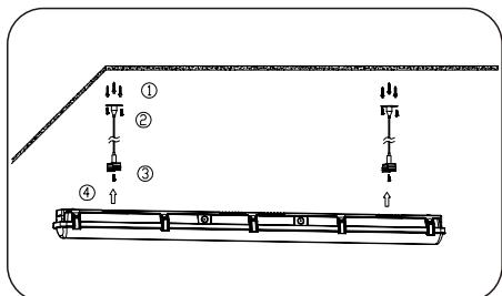
1. Secure suspended mounting kits to ceiling using 6-12 screws. Secure another side of suspended mounting kits to clips using 4-8 screws. Orient the luminaire so conduit fitting faces incoming supply power or conduit. Align the recesses and apply gentle upward pressure to secure luminaire onto both mounting clips.
