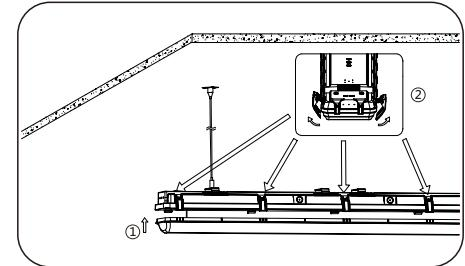
6. After align lens and bottom housing, turn off the luminaire. Secure lens to housing with lens latches.
