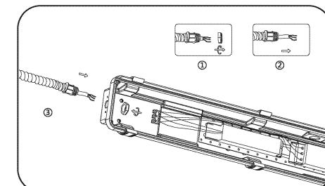
3. Disconnect the wire connecting the LED board and the driver to avoid unstable connection due to heavy suspension.
