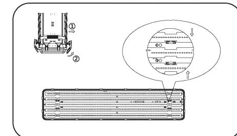
1. Secure mounting clips to ceiling using 4-8 screws. Space the clips 33.67 inches apart for 4 foot luminaire, or 37.8 inches apart for 8 foot luminaire. Orient the luminaire so conduit fitting faces incoming supply power or conduit. Align the recesses and apply gentle upward pressure to secure luminaire onto both mounting clips.
