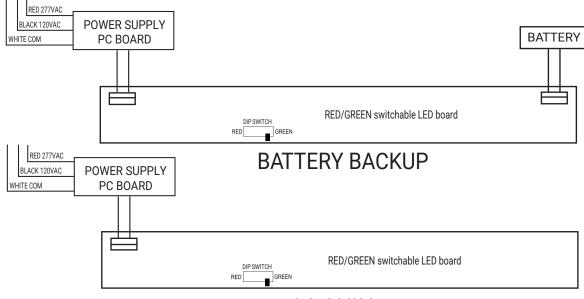
NOTE: Properly insulate the unused lead with a wire nut or other approved means. WARNING: Unused wires must be capped using enclosed wire nuts.
