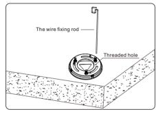
Screw the threaded end of the wire fixing rod into the corresponding threaded hole on the Mounting Base (tighten fully or to a proper position).
