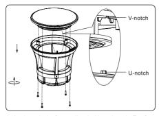
4. As shown in the figure, align the V-notch on the Top Cap with the U-notch on the Top Head, reinstall the Top Cap to its original position, and tighten the Hex socket screws.
