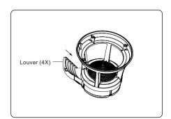
As shown in the figure, align one end of the Louver with the slot inside the Top Head
