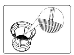
As shown in the figure, place the Diffuse Lens inside the Top Head.
