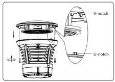
4. As shown in the figure, after installing the four Louvers, align the V-notch on the Top Cap with the U-notch on the Top Head, reinstall the Top Cap to its original position, and then tighten the Hex socket screws.
