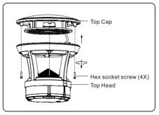
Remove the Hex socket screws from the Top Cap, then detach the Top Cap from the Top Head. During operation, do not overstretch the wires connected to the Top Cap to avoid poor electrical contact.
