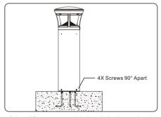
6. Install four screws, and the installation is completed.
