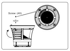
As shown in the figure, after ensuring the Louver is placed inside the Top Head, fasten the Louver with screw.
