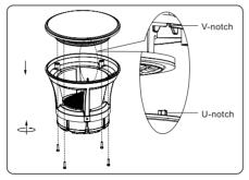
As shown in the figure, align the V-notch on the Top Cap with the U-notch on the Top Head, reinstall the Top Cap to its original position, and tighten the Hex socket screws.
