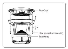
Remove the Hex socket screws from the Top Cap, then detach the Top Cap from the Top Head. During operation, do not overstretch the wires connected to the Top Cap to avoid poor electrical contact.
