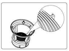
3. As shown in the figure, place the 180 Degree Glare Shield inside the Top Head.
