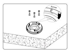
Adjust the position of the Mounting Base so that the direction of the arrow on it corresponds to the predefined Light Distribution Direction, then tighten the nuts on the Mounting Base.
