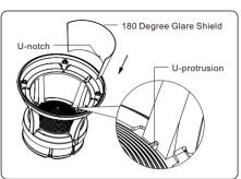
As shown in the figure, align the U-notch of the 180
