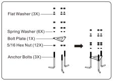
1.Install the anchor bolt assembly.
