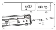
6. Separate the waterproof plug, and connect the input wire to the output wire of the driver after passing through the plug and outlet as shown in the figure.
