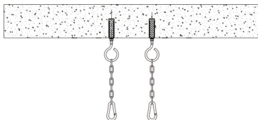
Step 3: Install Ø4 size stainless steel circular chain on the hooks
